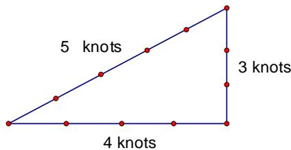
Using ropes that had knots that where equality spaced, the Egyptians could measure out right angles by making a 3-4-5 right angle or other right triangles with the rope.
