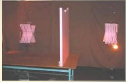
Power source and capture device suspended in mid-air about 2.5 meters apart with nylon thread
