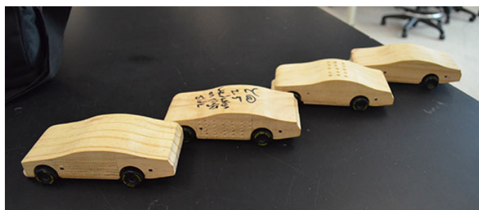
Above: Wooden cars with the dimples that Brian used in his wind tunnel studies.
