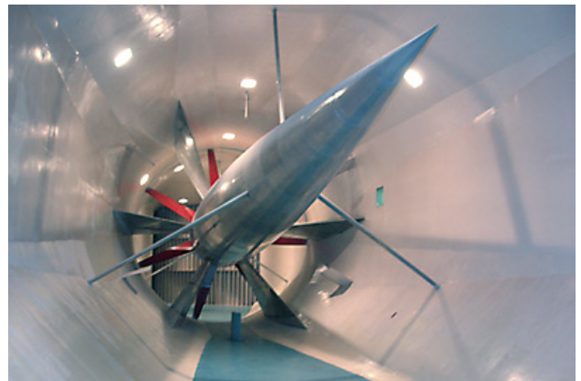
A large axial flow fan. Notice the stators just upstream of the fan blades. (6)
