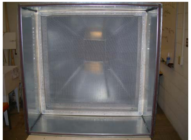
Settling chamber with both screens installed
