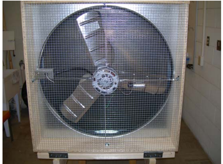
View of the fan mounted on the wind tunnel. Heavy gauge wire mesh is stapled to the frame to prevent debris from getting sucked in.
