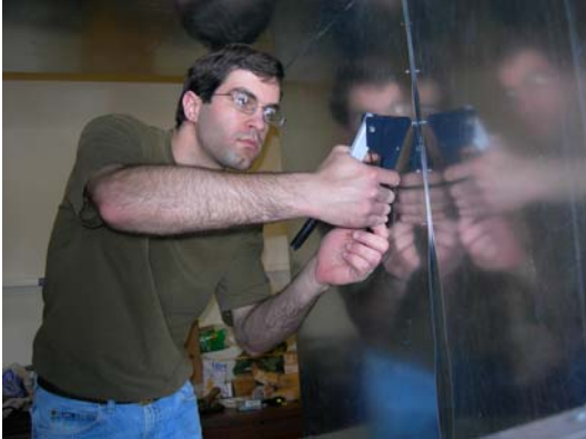
Riveting the settling chamber to the contraction section.
