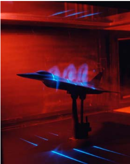
Smoke passing over a scale model airframe illuminated by lasers. (8)
