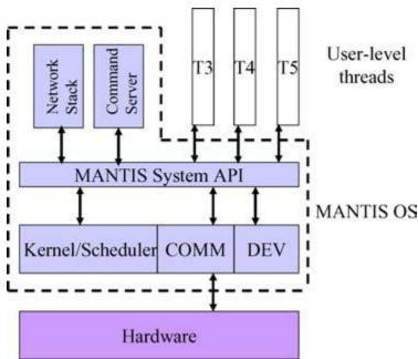
"MANTIS OS architecture compresses a classic multithreaded layered operating system design into <500 bytes of RAM."
