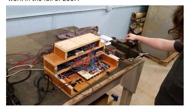
This was based on an Arduino microcontroller, a couple of multiplexers, sixteen 4-channel relays, sixteen copper electrodes and their connecting wires, and a conglomeration of shorter control wires that made everyone who saw it wince in pain! All of this directed the electrical current from a 120-volt ac generator through two relays at a time, with a voltage difference being measured via two other relay-activated electrodes.
