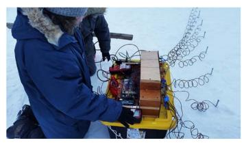
The goal of this was to recreate a small-scale galvanic resistivity array that could obtain data close to the surface to yield an electrical resistivity profile of the ice. Once again, after several attempts, fixes, and frustrations, it finally worked and did give that almost-magical cross section of the frighteningly-thin sea ice. Due to the extreme time crunch in getting ready for the trip, the current and voltage measurements were obtained manually with multimeters.
